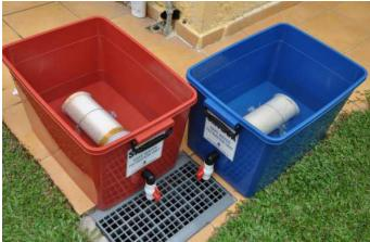
Photo 1.0 / 2.0: locally sourced storage containers were adapted for the SkyBox™ membrane
